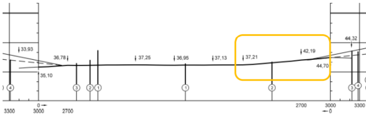
Figure 4: Typical example of 'complex mean LSAA slope greater than 0.8% but lower than 1%' (EDD 23L dated 2009)
